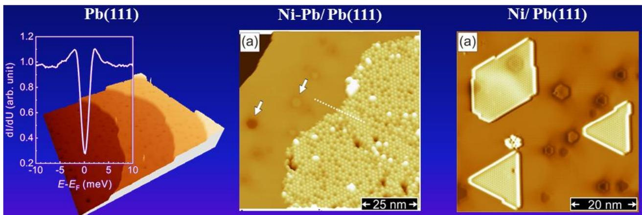
**Figure:** Superconducting gap measured at the pristine Pb(111) substrate (**Left**). STM topography of monatomic Ni-Pb surface alloy on Pb(111) by means of high temperature growth (**Middle**). In contrast, honeycomb-structured Ni nanoislands can be fabricated on Pb(111) by low temperature deposition (**Right**).
