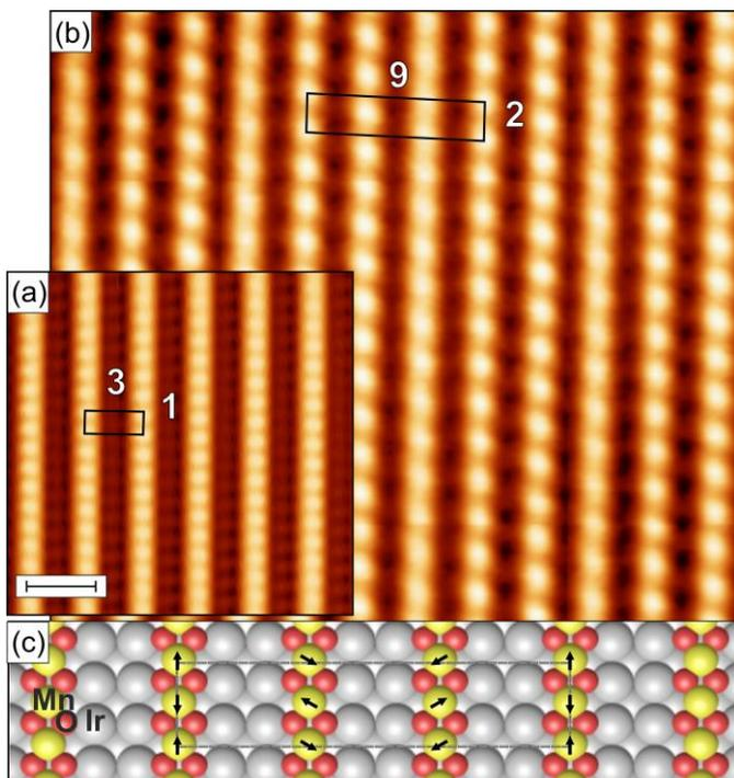
**Figure:** Atomic resolution scans of MnO<sub>2</sub> chains on Ir(001). (a) A  $(3 \times 1)$  structural unit cell is observed with a non-magnetic W tip (scale bar: 1 nm). (b) With a Cr-coated W tip the magnetic  $(9 \times 2)$  unit cell is resolved. (c) Schematic model of the chiral  $(9 \times 2)$  spin structure of MnO<sub>2</sub>/Ir(001).
