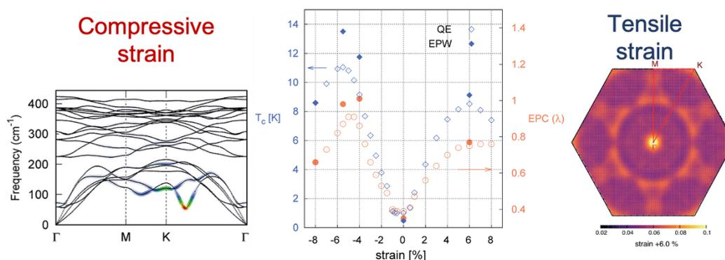
**Figure:** Calculation results in Li-intercalated bilayer MoS<sub>2</sub> (**Left**) electron-phonon interaction projected on phonon band structure under 5.5% compressive strain (**Middle**)  $T_c$  as a function of strain (**Right**) nesting function under 6% tensile strain.
