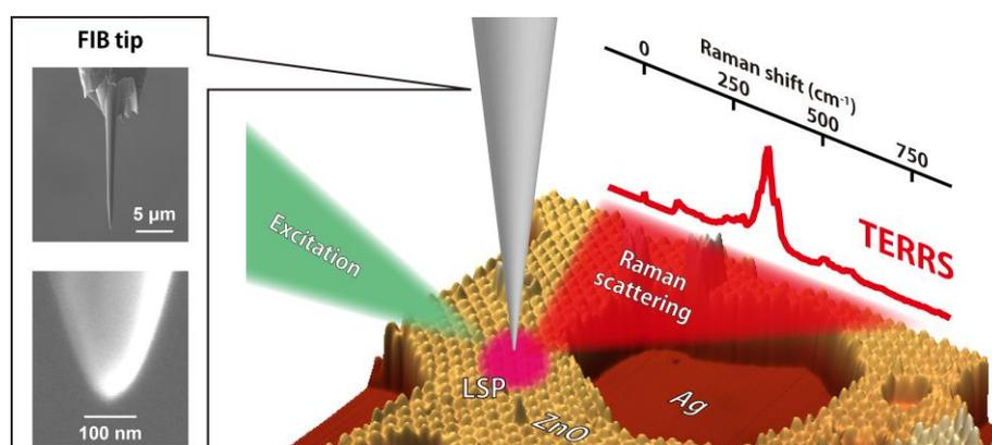
**Resolving the Correlation between Tip-Enhanced Resonance Raman Scattering and Local Electronic States of ultrathin zinc oxide films with 1 nm Resolution [2].**
